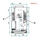
**CONNECTIONS** E = ELECTRIC D = DRAIN
